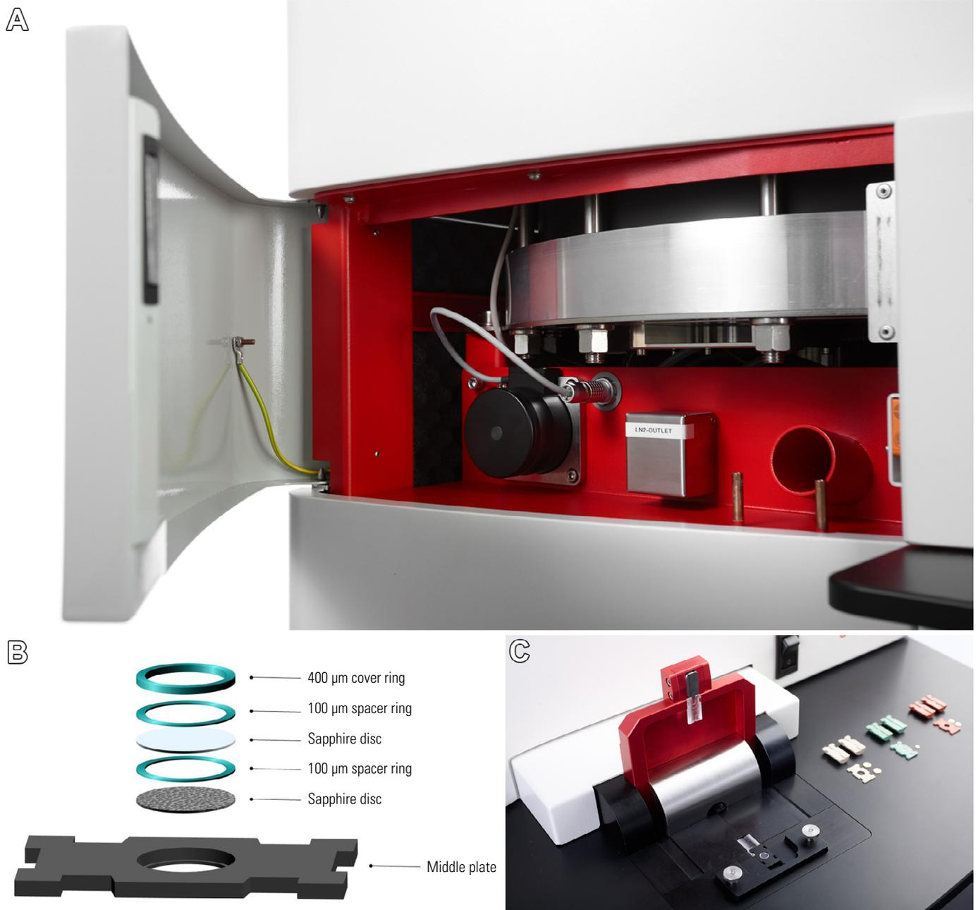
Fig. 3: A) Insertion of the light module into the socket at the front of the instrument. B) Loading of the sapphire sandwich for light stimulation. C) Shifting the middle plate on the transparent half cylinder (black surface).
