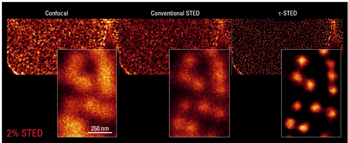
Figure 3:  $\tau$ -STED 660 at extremely low STED power on COS7 cells immunostained for nuclear pores (NUPs). The primary antibody recognizes several proteins of the nuclear pore basket, so the NUPs are labeled in the central region and as a result they appear as point-like structures in the images.
